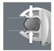
The parallel, smooth jaws of the 7880 Joker offer a seating stress and can thus prevent the nut or screw head from rounding, which can occur when power is transmitted over corners.
